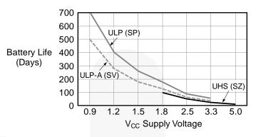
Figure 1. Battery Life vs. Vcc Supply Voltage
