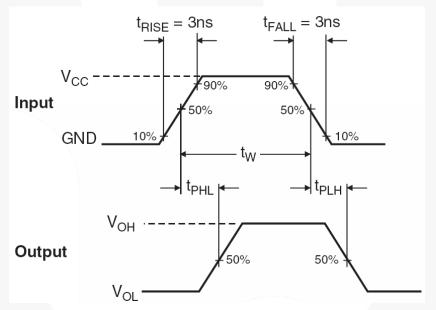
Figure 6. AC Waveforms
