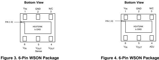
Figure 4. 6-Pin WSON Package Adjustable Output Voltage See Package Number NGD0006A
