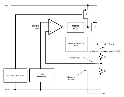
Figure 22. LP8340 Functional Block Diagram
