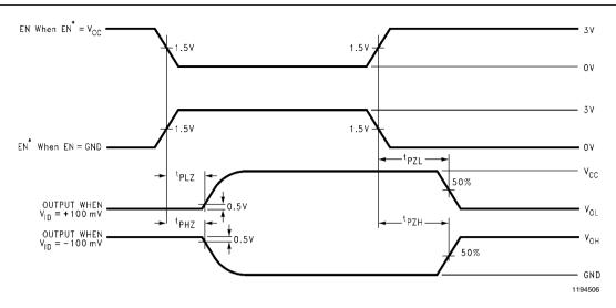
FIGURE 4. Receiver TRI-STATE Delay Waveforms
