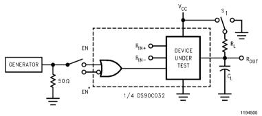
$\mathbf{C}_{\mathbf{L}}$  includes load and test jig capacitance.
