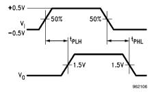
$V_i$ Amplitude: 1.0V Offset: 0.5V Pulse Width: 100 ns PRR: 5.0 MHz  $t_r = t_f \leq 5.0$  ns
