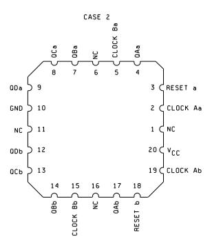
FIGURE 1. Terminal connections.
