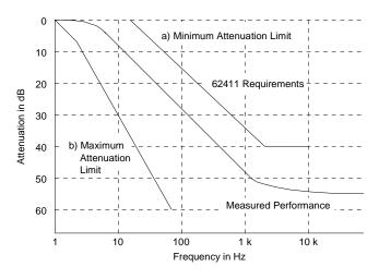
**Figure 12. Typical Jitter Transfer Function**
