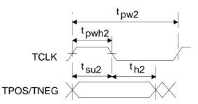
Figure 3. Transmit Clock and Data Switching Characteristics
