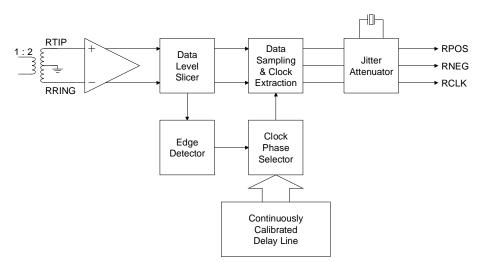
Figure 10. Receiver Block Diagram
