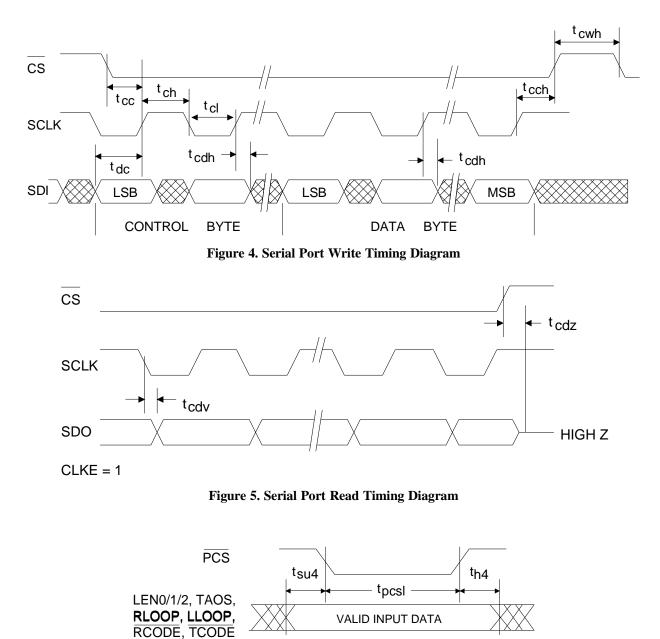
Figure 6. Extended Hardware Mode Parallel Chip Select Timing Diagram
