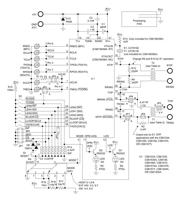
Figure 1. Evaluation Board Schematic
