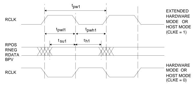
Figure 2. Recovered Clock and Data Switching Characteristics
