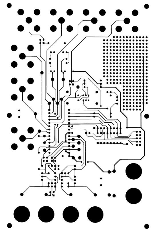
Figure 4. Bottom Trace Layer (NOT TO SCALE)
