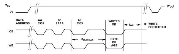
FIGURE 6. TIMING SEQUENCE—BYTE OR PAGE WRITE
