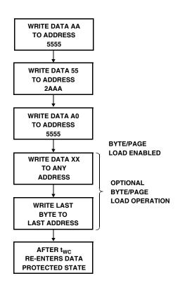
Regardless of whether the device has previously been protected or not, once the software data protection algorithm is used and data has been written, the X28HC256 will automatically disable further writes unless another command is issued to cancel it. If no further commands are issued the X28HC256 will be write protected during power-down and after any subsequent power-up.
