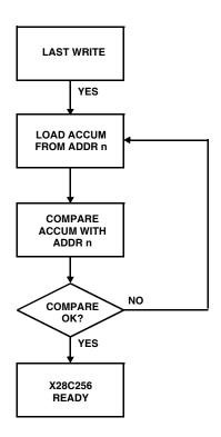
FIGURE 5. TOGGLE BIT SOFTWARE FLOW
