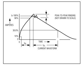
Figure 7. Human Body Model Current Waveform
