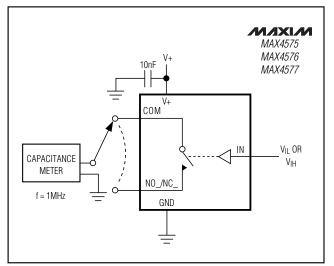
Figure 4. Channel Off/On-Capacitance
