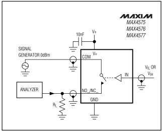
Figure 2. Off-Isolation/On-Channel Bandwidth
