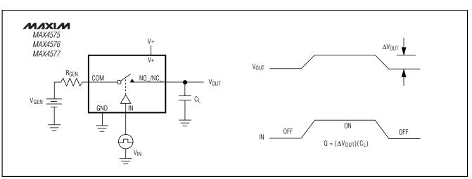
Figure 3. Charge Injection
