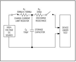
Figure 8. IEC 1000-4-2 ESD Test Model
