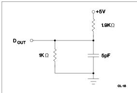
Figure 4. Output Load A
