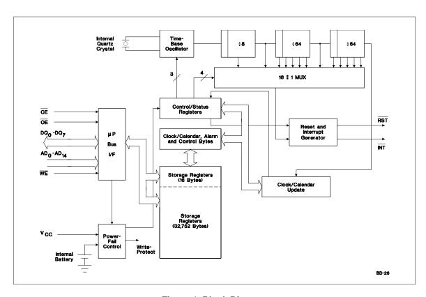
Figure 1. Block Diagram
