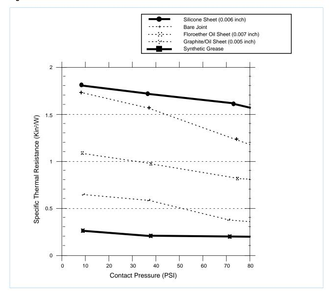
The board designer can choose between several types of thermal interfaces. Heat sink adhesive materials should be selected based upon high conductivity, yet adequate mechanical strength to meet equipment shock/vibration requirements. There are several commercially-available thermal interfaces and adhesive materials provided by the following vendors.
