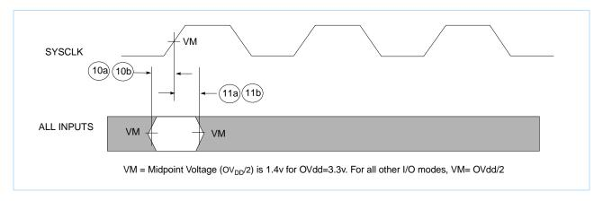
Figure 4 provides the mode select input timing diagram for the PID8p-750.
