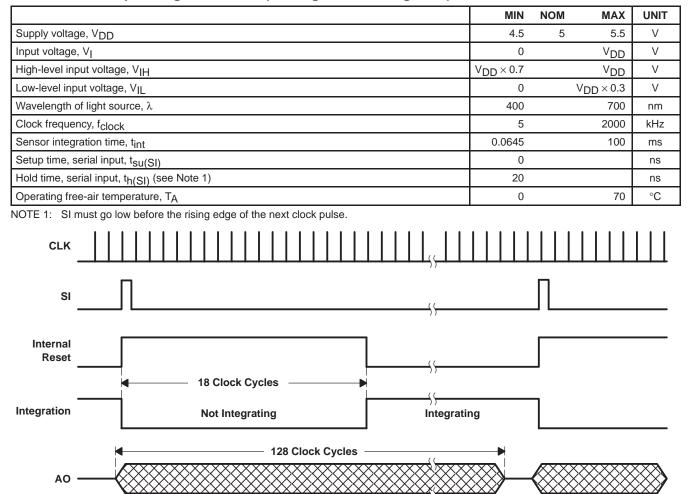
Figure 1. Timing Waveforms
