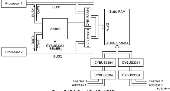
Figure 7. High Speed Dual Port RAM
