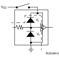
Figure 6. Gate Input (Power OFF)
