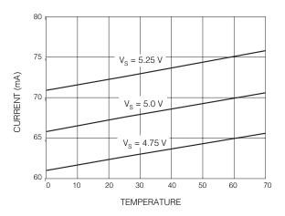
Fig. 3 Supply Current vs Temperature
