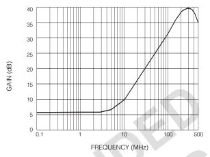
Fig. 4 Equalizer Gain vs Frequency
