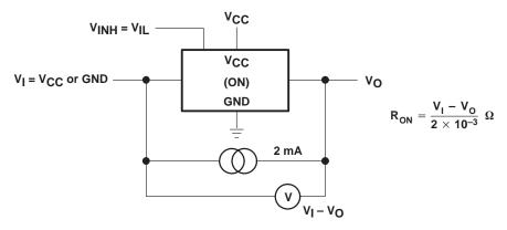
Figure 1. On-State Resistance Test Circuit
