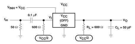
Figure 9. Feed-Through Attenuation (Switch Off)
