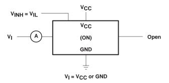
Figure 3. On-State Switch Leakage-Current Test Circuit
