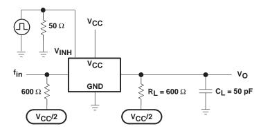
Figure 8. Crosstalk Between Control Input and Switch Output
