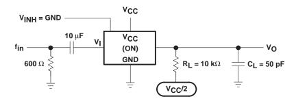
Figure 10. Sine-Wave Distortion
