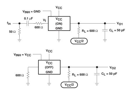
Figure 7. Crosstalk Between Any Two Switches
