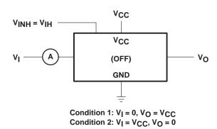
Figure 2. Off-State Switch Leakage-Current Test Circuit
