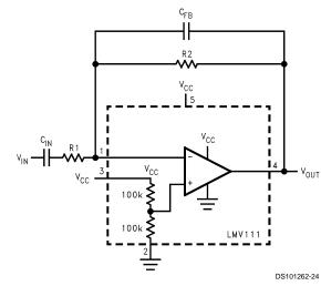
FIGURE 2. Phase Inverting AC Amplifier
