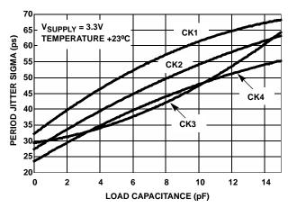
FIGURE 1. STANDARD DEVIATION vs LOAD CAPACITANCE
