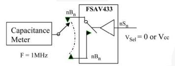
Figure 16. Channel Off Capacitance
