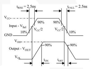
Figure 10. Turn On / Off Waveforms
