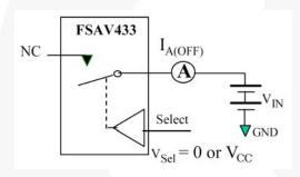
Figure 9. Off Leakage
