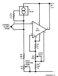
$200^{\circ}C{\le}T_p{\le}700^{\circ}C$ 1 mA≤l<sub>OUT</sub>≤5 mA †Gain Trim
