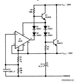
$$V_{OUT} = \frac{R2}{R1} V_{REF}$$
