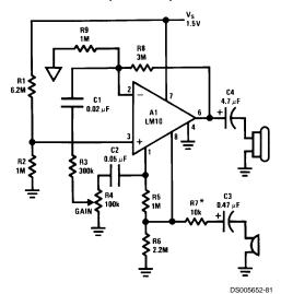
$Z_{OUT}$ -680 $\Omega$  @ 5 kHz  $A_V \le 1$ k  $f_1$ -100 Hz  $f_2$ -5 kHz  $R_L \sim 500$  \*Max Gain Trim
