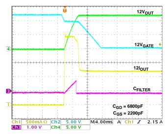
FIGURE 5. 12VMAIN START-UP RLOAD =  $10\Omega$ ,  $C_{LOAD} = 470 \mu F$
