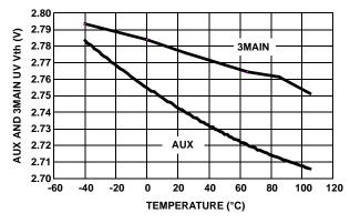
FIGURE 29. AUX AND 3MAIN POWER GOOD THRESHOLD VOLTAGE vs TEMPERATURE
