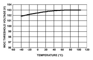
FIGURE 23. FAST TRIP THRESHOLD VOLTAGE vs TEMPERATURE
