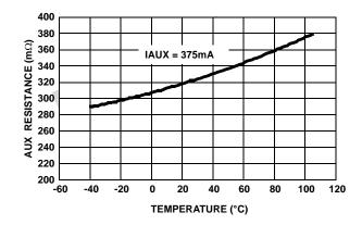
FIGURE 25. AUX  $r_{DS(ON)}$  vs TEMPERATURE
