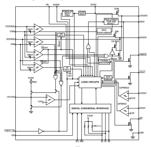
BOTH A AND B SLOTS SHARE THE SCL, SDA, A0, A1, A2,  $\overline{\text{INT}}$  PINS.
