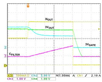
FIGURE 9. 3VMAIN CR AND SHUT-DOWN
