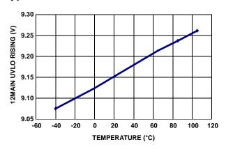
FIGURE 26. 12MAIN RISING UVLO THRESHOLD VOLTAGE VS TEMPERATURE
