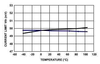
FIGURE 22. CURRENT LIMIT THRESHOLD VOLTAGE vs TEMPERATURE
