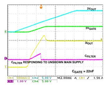
FIGURE 4. 3VMAIN START-UP  $R_{LOAD}$  =  $2\Omega$ ,  $C_{LOAD}$  =  $470\mu F$
