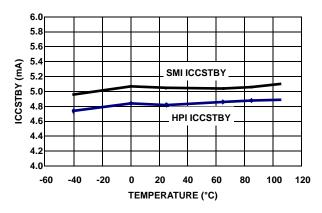
FIGURE 20. ICCSTBY CURRENT vs TEMPERATURE
