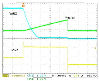
FIGURE 13. VAUX WOC REGULATION AND SHUT-DOWN
