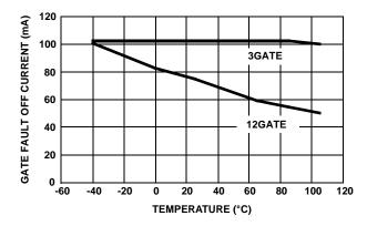
FIGURE 31. GATE FAULT OFF CURRENT (ABS) vs TEMPERATURE
