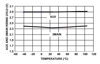
FIGURE 27. AUX AND 3.3MAIN RISING UVLO THRESHOLD VOLTAGE vs TEMPERATURE
