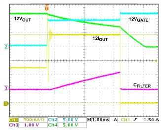
FIGURE 8. 12VMAIN CR AND SHUT-DOWN
