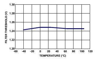
FIGURE 33. FILTER THRESHOLD VOLTAGE vs TEMPERATURE
