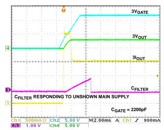
FIGURE 6. 3VMAIN START-UP RLOAD = 2 $\Omega$ , CLOAD = 470 $\mu$ F
