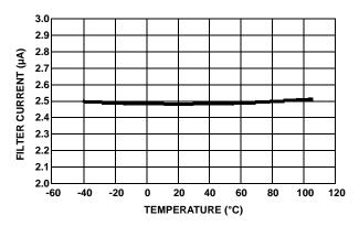
FIGURE 32. FILTER CHARGE CURRENT vs TEMPERATURE
