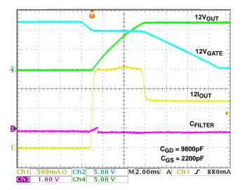
FIGURE 7. 12VMAIN START-UP  $R_{LOAD} = 10\Omega$ ,  $C_{LOAD} = 470 \mu F$
