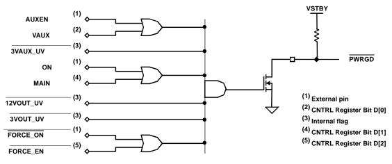
FIGURE 14. PWRGD LOGIC DIAGRAM
