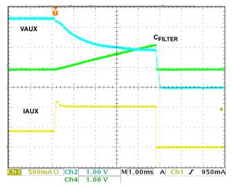
FIGURE 12. VAUX OC REGULATION AND SHUT-DOWN
