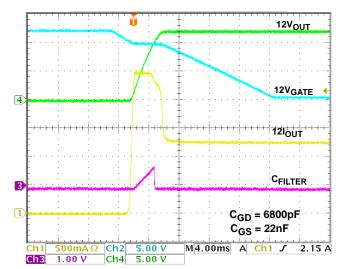
FIGURE 3. 12VMAIN START-UP  $R_{LOAD} = 10\Omega$ ,  $C_{LOAD} = 470 \mu F$
