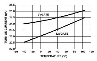
FIGURE 30. ISL6112 GATE TURN-ON CURRENT (ABS) vs TEMPERATURE
