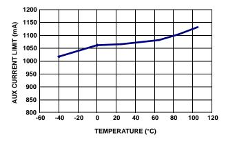
FIGURE 24. AUX. CURRENT LIMIT vs TEMPERATURE
