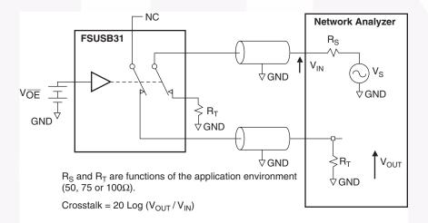
Figure 18. Non-Adjacent Channel-to-Channel Crosstalk
