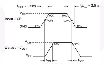
Figure 13. Turn On / Turn Off Waveform ( $t_{ON}$  /  $t_{OFF}$ )
