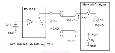
Figure 17. Channel Off Isolation
