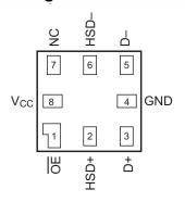
Figure 3. Pin Assignments for MicroPak
