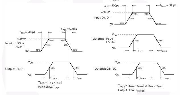
Figure 15. Switch Skew Tests
