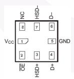
Figure 5. Pin Assignments for UMLP
