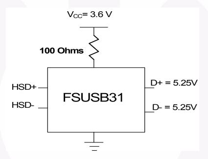
Figure 21. A 100 $\Omega$  resistor in series with the V<sub>CC</sub> supply allows the FSUSB31 to withstand a Vbus short when powered up
