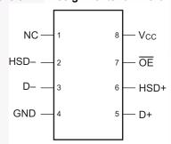
Figure 4. Pin Assignments for US8
