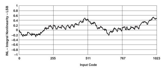
Figure 16. Integral Nonlinearity With Input Code
