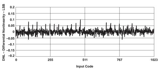
Figure 15. Differential Nonlinearity With Input Code
