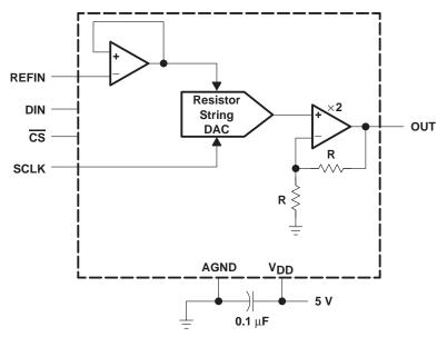
Figure 17. TLC5617 Typical Operating Circuit
