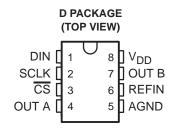
The TLC5617 and TLC5617A are dual 10-bit voltage output digital-to-analog converters (DAC) with buffered reference inputs (high impedance). The DACs have an output voltage range that is two times the reference voltage, and the DACs are monotonic. The devices are simple to use, running from a single supply of 5 V. A power-on reset function is incorporated to ensure repeatable start-up conditions.
