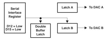
Figure 20. Latch B and Double-Buffer Write
