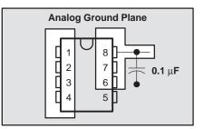
Figure 26. Power-Supply Bypassing
