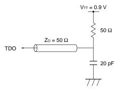
JTAG AC Characteristics (T<sub>A</sub> = 0 to 70°C)
