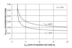
Figure 4. On-Resistance Variation with Gate-to-Source Voltage.
