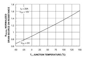
Figure 3. On-Resistance Variation with Temperature.
