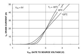
Figure 5. Transfer Characteristics.
