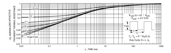
Figure 11. Transient Thermal Response Curve.
