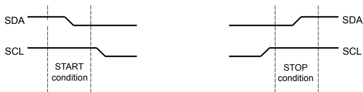
Figure 15-3. START and STOP Conditions
