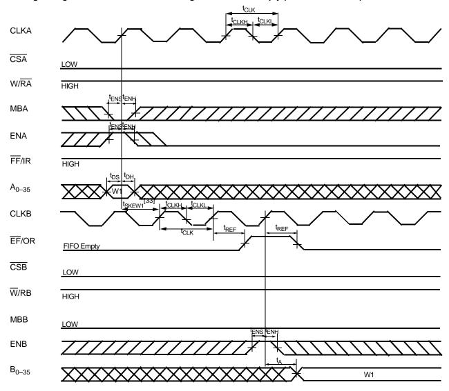
33. t<sub>SKEW1</sub> is the minimum time between a rising CLKA edge and a rising CLKB edge for EF to transition HIGH in the next CLKB cycle. If the time between the rising CLKA edge and rising CLKB edge is less than t<sub>SKEW1</sub>, then the transition of EF HIGH may occur one CLKB cycle later than shown.
