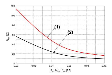
Figure 6. R<sub>SC</sub> Variation by Change of Shunt Resistors ( R<sub>SU</sub>, R<sub>SV</sub>, R<sub>SW</sub>) for Short-Circuit Protection (1) @ Current Trip Level ≒ 15.0 A (2) @ Current Trip Level ≒ 22.5 A
