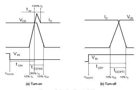
Figure 4. Switching Time Definition
