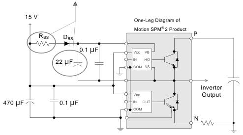
Figure 13. Recommended Bootstrap Operation Circuit and Parameters
