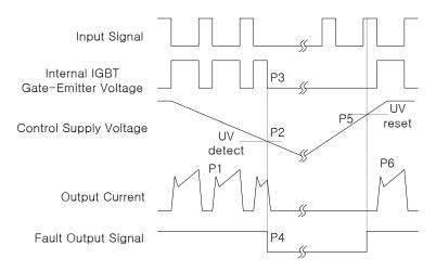
P1 : Normal operation: IGBT ON and conducting current .
