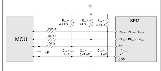
Figure 12. Recommended MCU I/O Interface Circuit
