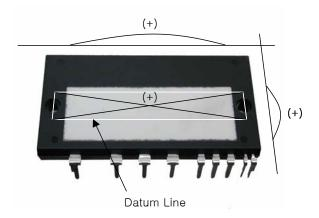
Figure 7. Flatness Measurement Position of The Ceramic Substrate
