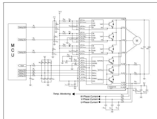
Figure 14. Application Circuit
