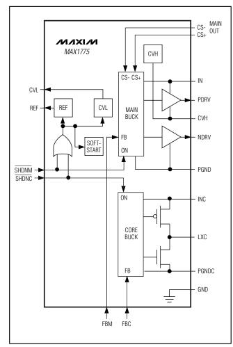
Figure 3. Simplified Block Diagram
