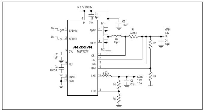
Figure 4. High Input Voltage Cascaded Configuration
