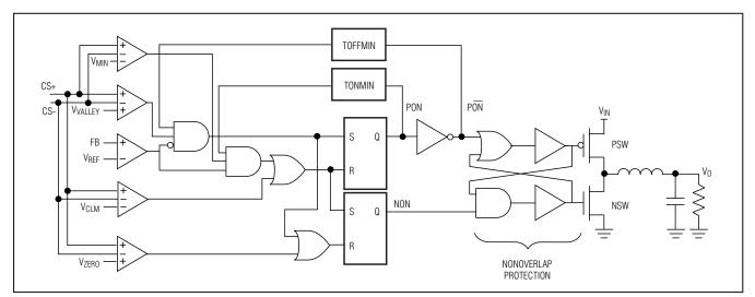
Figure 2. Simplified Control System Block Diagram
