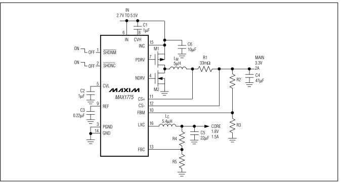
Figure 1. Typical Application Circuit (Low Input Voltage)
