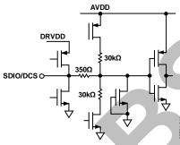
Figure 19. Equivalent SDIO/DCS Input Circuit
