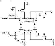
Figure 26. Switched Capacitor Input Circuit
