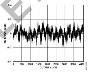
Figure 16. INL Error with  $f_{IN} = 9.7 \text{ MHz}$
