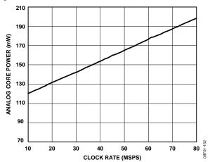
Figure 44. Analog Core Power vs. Clock Rate
