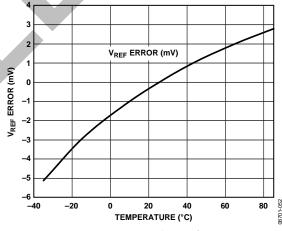
Figure 35. Typical V<sub>REF</sub> Drift
