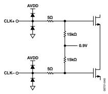
Figure 18. Equivalent Clock Input Circuit
