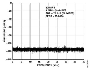
Figure 6. Single-Tone FFT with  $f_{IN} = 9.7$  MHz
