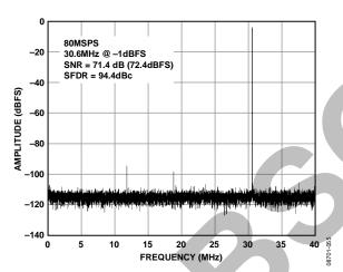
Figure 7. Single-Tone FFT with  $f_{IN} = 30.6 \, \text{MHz}$
