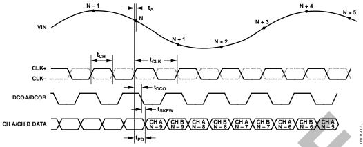
Figure 3. CMOS Interleaved Output Timing
