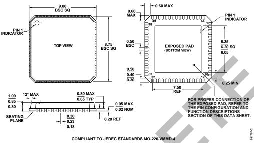
Figure 51. 64-Lead Lead Frame Chip Scale Package [LFCSP\_VQ] 9 mm × 9 mm Body, Very Thin Quad (CP-64-4) Dimensions shown in millimeters
