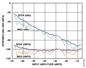
Figure 11. Two-Tone SFDR/IMD3 vs. Input Amplitude (AIN) with  $f_{IN1} = 28.3 \text{ MHz}$  and  $f_{IN2} = 30.6 \text{ MHz}$
