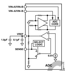
Figure 33. Internal Reference Configuration
