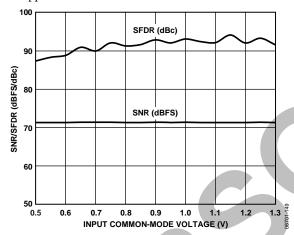
Figure 27. SNR/SFDR vs. Input Common-Mode Voltage,  $f_{IN} = 30.5$  MHz,  $f_S = 80$  MSPS
