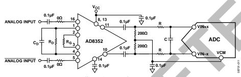
Figure 32. Differential Input Configuration Using the AD8352
