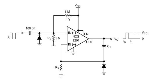
The resistor divider  $\mathsf{R}_1$  and  $\mathsf{R}_2$  can be used to set the magnitude of the input pulse. The pulse width is set by adjusting  $\mathsf{C}_1$  and  $\mathsf{R}_3.$
