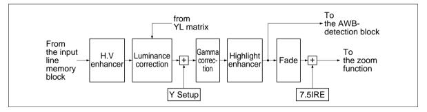
Figure 5 Luminance-Signal-Processing Block
