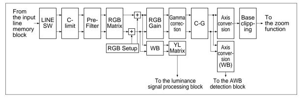
Figure 4 Color-Signal Processing Block
