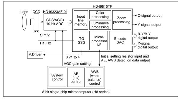
Figure 2 System Configuration
