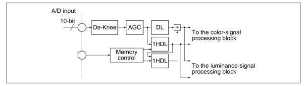
Figure 3 Input Line Memory Block
