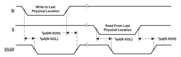
Figure 9. Expansion-Out Waveforms
