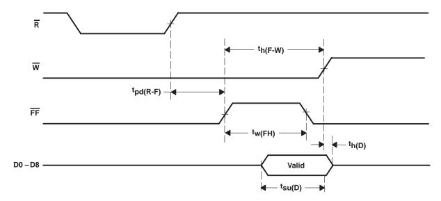
Figure 6. Automatic-Write Waveforms
