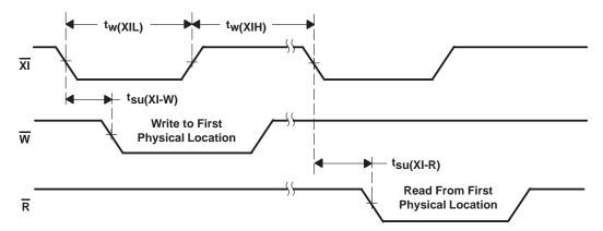
Figure 10. Expansion-In Waveforms
