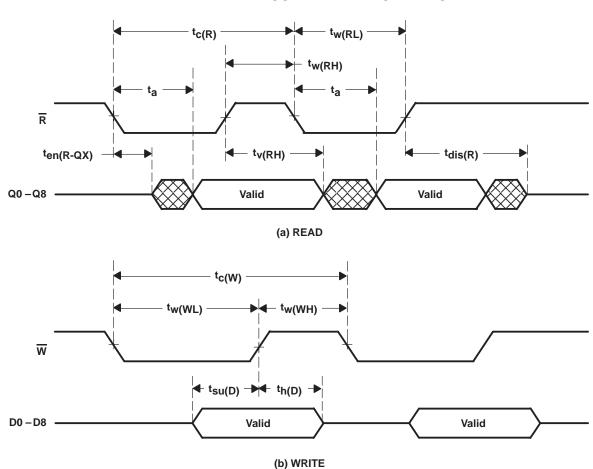
Figure 1. Asynchronous Waveforms
