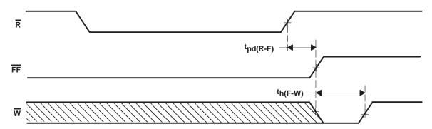
Figure 12. Minimum Timing for a Full-Flag Coincident-Write Pulse
