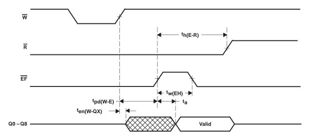
Figure 5. Automatic-Read Waveforms
