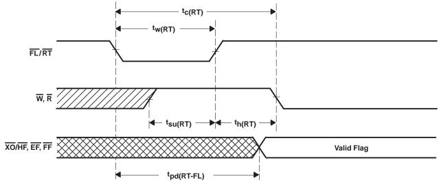
NOTE A: The  $\overline{\text{EF}}$ ,  $\overline{\text{FF}}$ , and  $\overline{\text{XO}}/\overline{\text{HF}}$  status flags are valid after completion of the retransmit cycle.
