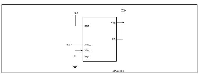
Figure 30.  $I_{DD}$  Test Condition, Power Down Mode All other pins are disconnected. V\_{DD}=2 V to 5.5 V
