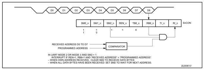
Figure 14. UART Multiprocessor Communication, Automatic Address Recognition
