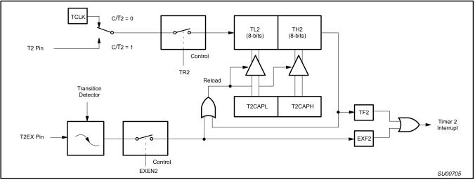
Figure 8. Timer 2 in Auto-Reload Mode (DCEN = 0)
