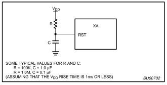
Figure 15. Recommended Reset Circuit
