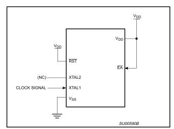
Figure 26. I<sub>DD</sub> Test Condition, Idle Mode All other pins are disconnected
