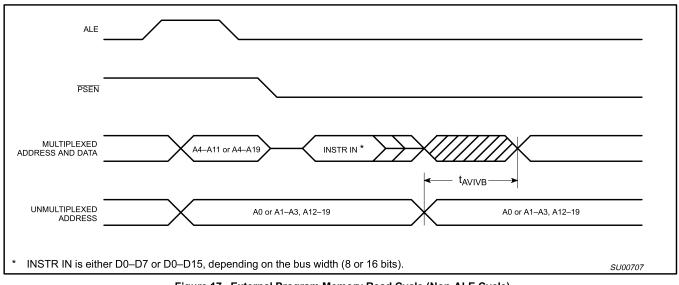
Figure 17. External Program Memory Read Cycle (Non-ALE Cycle)
