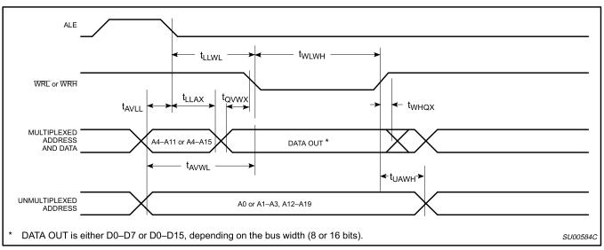
Figure 20. External Data Memory Write Cycle
