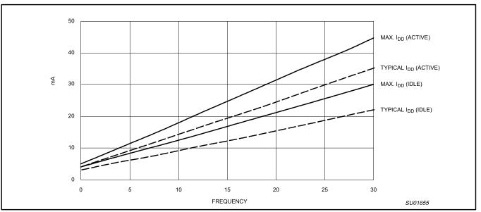
Figure 27.  $I_{DD}$  vs. Frequency at  $V_{DD}$  = 5.5 V
