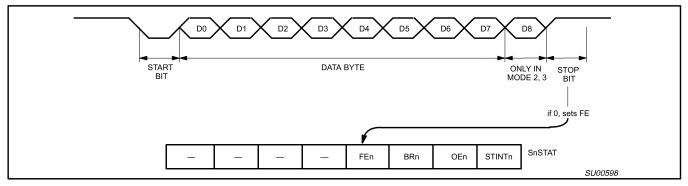
Figure 13. UART Framing Error Detection
