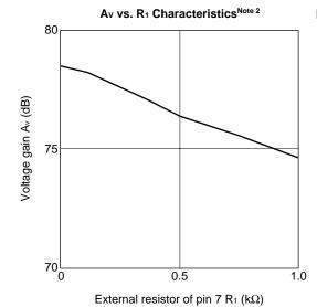
**Note 2.** This is the value of a resistor that is externally connected as follows:
