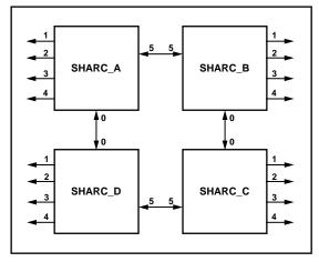
Figure 4. Link Port Connections
