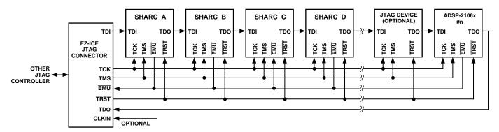
Figure 7. JTAG Scan Path Connections for the AD14160/AD14160L
