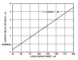
Figure 36. Typical Output Delay or Hold vs. Load Capacitance (at Maximum Case Temperature)  $(V_{DD} = 3.3 \text{ V})$
