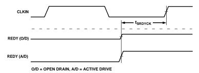
Figure 19a. Synchronous REDY Timing
