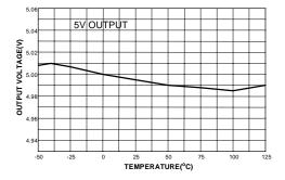
Figure 5. Output Voltage vs. Temperature
