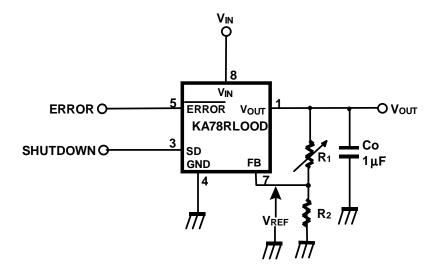
$V_0 = V_{REF} (1 + R_1/R_2) + I_{FB} R_1$
