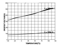
Figure 7. Dropout Voltage
