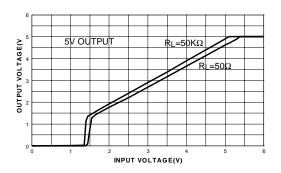
**Figure 2. Dropout Characteristics**
