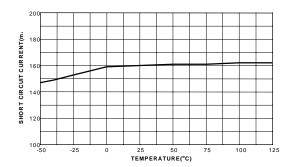
**Figure 6. Short Circuit Current**
