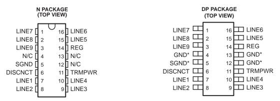
\* DP package pin 5 serves as signal ground; pins 4, 12, 13 serve as heatsink/ground.
