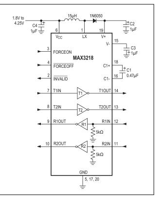
Figure 1. Typical Operating Circuit
