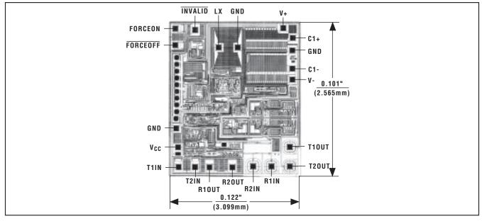
TRANSISTOR COUNT: 571 SUBSTRATE CONNECTED TO GND
