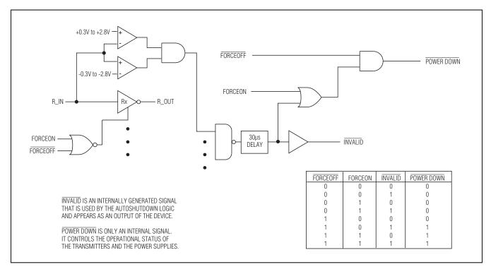
Figure 3. AutoShutdown Logic
