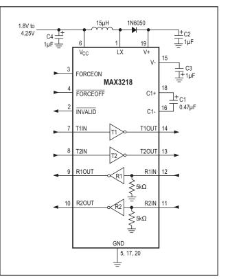
Figure 1. Typical Operating Circuit
