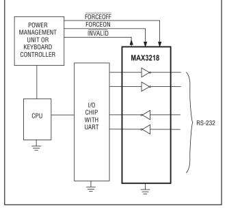
Figure 2. Interface Under Control of PMU
