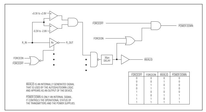
Figure 3. AutoShutdown Logic
