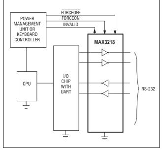
Figure 2. Interface Under Control of PMU
