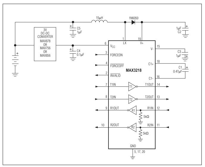
Figure 6. Operating from Unregulated and Regulated Supplies
