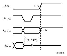
FIGURE 6. Loss of Lock
