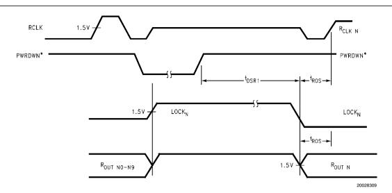
FIGURE 4. Locktime from PWRDNn t<sub>DSR1</sub>
