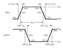
FIGURE 3. AC Waveforms
