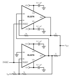
INVERTING 200mA OUTPUT CURRENT DISTRIBUTION AMPLIFIER
