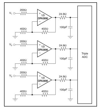
Figure 43. Triple ADC Driver
