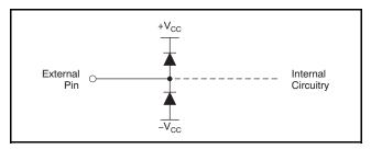
Figure 54. Internal ESD Protection
