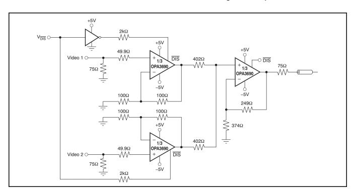
Figure 44. Buffered 2 x 1 Multiplexer
