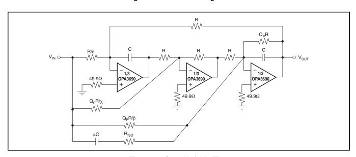
Figure 46. State Variable Filter
