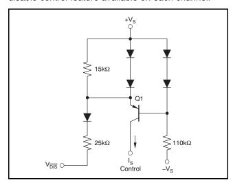
Figure 52. Simplified Disable Control Circuit
