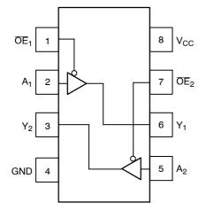
Figure 1. Pinout (Top View)
