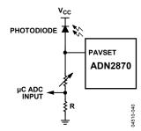
Figure 31. Single Measurement of I<sub>MPD</sub> Across a Sense Resistor in Resistor Setpoint I<sub>MPD</sub> Monitoring
