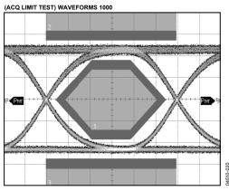
Figure 20. Optical Eye 155 Mbps, 1.078 ns/DIV, PRBS 2<sup>31-1</sup>, PAV = -4.5 dBm, ER = 9 dB, Mask Margin 50%
