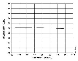
Figure 15. IMOD/IMMON Gain vs. Temperature, I<sub>MOD</sub> = 30 mA
