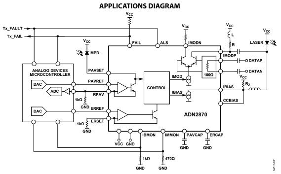
Figure 1. Application Diagram Showing Microcontroller Interface
