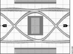
Figure 22. Optical Eye 2.488 Gbps, 65 ps/DIV, PRBS  $2^{31-1}$ , PAV = -0.2 dBm, ER = 8.96 dB, Mask Margin 21%, T<sub>A</sub> = 85°C
