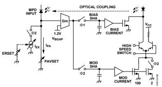
Figure 24. Dual-Loop Control of Average Power and Extinction Ratio
