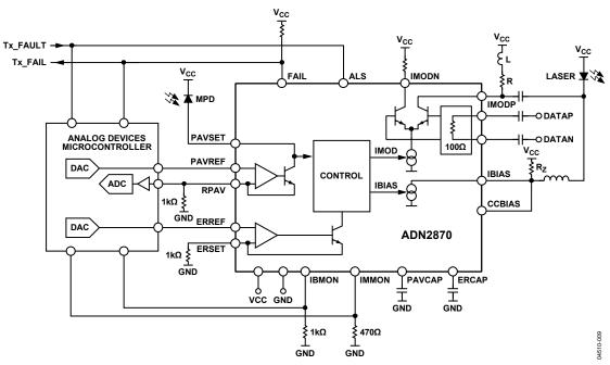
Figure 26. Using MicroConverter Calibration and Monitoring
