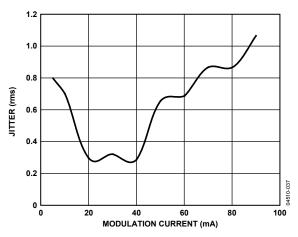
Figure 9. Random Jitter vs. Modulation Current, I<sub>BIAS</sub> = 20 mA
