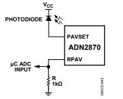
Figure 28. Single Measurement of I<sub>MPD</sub> at RPAV in Voltage Setpoint Mode
