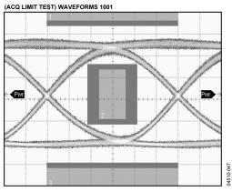
Figure 21. Optical Eye 2.488 Gbps, 65 ps/DIV, PRBS  $2^{31-1}$ , PAV = 0 dBm, ER = 9 dB, Mask Margin 22%, T<sub>A</sub> = 25°C
