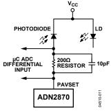
Figure 29. Differential Measurement of I<sub>MPD</sub> Across a Sense Resistor
