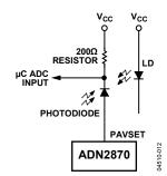
Figure 30. Single Measurement of I<sub>MPD</sub> Across a Sense Resistor
