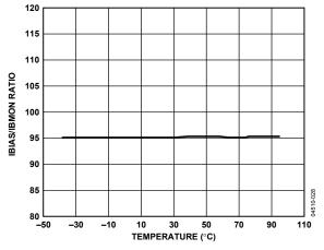
Figure 12. IBIAS/IBMON Gain vs. Temperature, I<sub>BIAS</sub> = 20 mA
