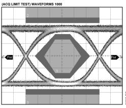
Figure 19. Optical Eye 622 Mbps, 264 ps/DIV, PRBS 2<sup>31-1</sup>, PAV = -4.5 dBm, ER = 9 dB, Mask Margin 50%
