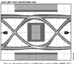
Figure 18. Optical Eye 2.488 Gbps, 65 ps/DIV, PRBS 2<sup>31-1</sup>, PAV = -4.5 dBm, ER = 9 dB, Mask Margin 25%
