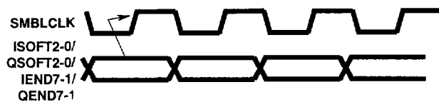
FIGURE 19. OUTPUT DATA CLOCK TIMING
