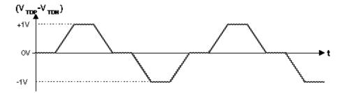
The magnetics module external to the 82562EZ converts  $I_{TDP}$  and  $I_{TDN}$  to  $2.0~V_{PP}$ , as required by the TP-PMD specification. The same magnetics used for 100BASE-TX mode can also work in 10BASE-T mode.
