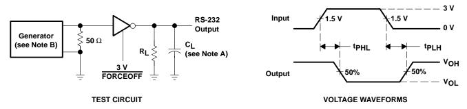
NOTES: A. C<sub>I</sub> includes probe and jig capacitance.
