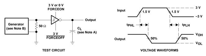
NOTES: C. C<sub>I</sub> includes probe and jig capacitance.
