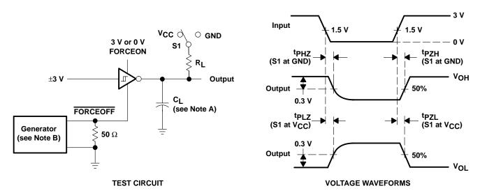
NOTES: A. C<sub>I</sub> includes probe and jig capacitance.
