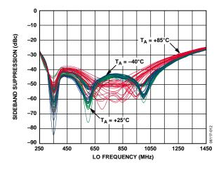
Figure 12. Sideband Suppression vs.  $f_{L0}$  and Temperature Multiple Devices Shown
