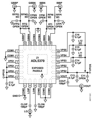
Figure 36. ADL5370 Evaluation Board Schematic
