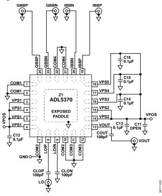
Figure 25. Basic Connections for the ADL5370
