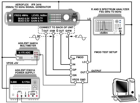
Figure 38. Characterization Bench Setup
