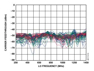
Figure 10. Carrier Feedthrough vs. f<sub>LO</sub> and Temperature Multiple Devices Shown
