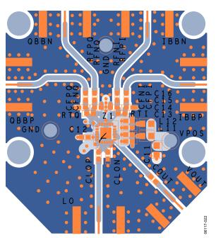
Figure 37. Evaluation Board Layout, Top Layer
