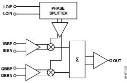
Figure 24. Block Diagram
