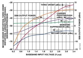
Figure 15. Second- and Third-Order Distortion, Carrier Feedthrough, Sideband Suppression, and SSB  $P_{OUT}$  vs. Baseband Differential Input Level ( $f_{LO} = 900 \text{ MHz}$ )
