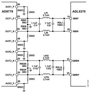
Figure 33. DAC Modulator Interface with Auxiliary DAC Resistors
