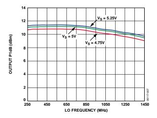
Figure 7. SSB Output 1 dB Compression Point (OP1dB) vs. f<sub>LO</sub> and Supply
