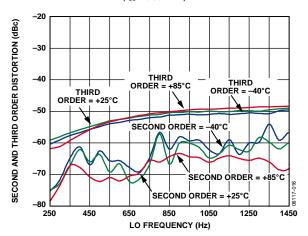
Figure 16. Second- and Third-Order Distortion vs. f<sub>LO</sub> and Temperature (Baseband I/Q Amplitude = 1.4 V p-p differential)
