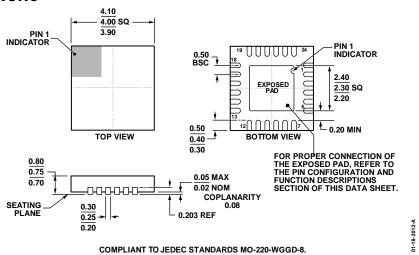
Figure 40. 24-Lead Lead Frame Chip Scale Package [LFCSP] 4 mm × 4 mm Body, and 0.75 mm Package Height (CP-24-14) Dimensions shown in millimeters
