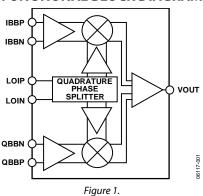
The ADL5370 accepts two differential baseband inputs and a single-ended LO and generates a single-ended 50  $\Omega$  output.
