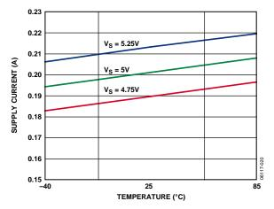
Figure 22. Power Supply Current vs. Temperature
