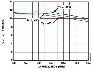
Figure 6. SSB Output 1 dB Compression Point (OP1dB) vs. f<sub>LO</sub> and Temperature
