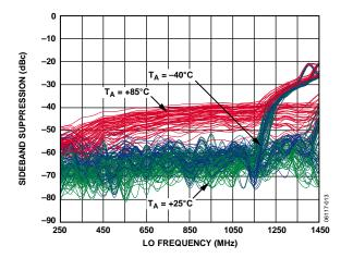
Figure 13. Sideband Suppression vs. f₁o and Temperature after Nulling at 25℃ Multiple Devices Shown
