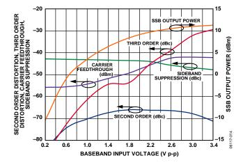
Figure 14. Second- and Third-Order Distortion, Carrier Feedthrough, Sideband Suppression, and SSB  $P_{OUT}$  vs. Baseband Differential Input Level ( $f_{LO} = 450 \text{ MHz}$ )
