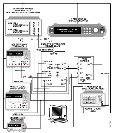
Figure 39. Setup for Baseband Frequency Sweep and Undesired Sideband Nulling
