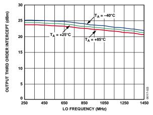
Figure 18. OIP3 vs. Frequency and Temperature
