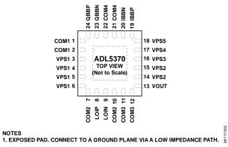
Figure 2. Pin Configuration
