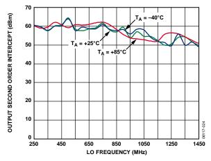
Figure 19. OIP2 vs. Frequency and Temperature
