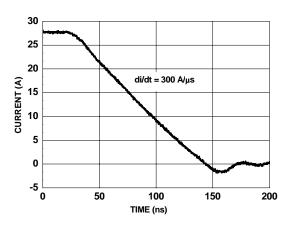
Figure 14. FDMS0343S SyncFET body diode reverse recovery characteristic
