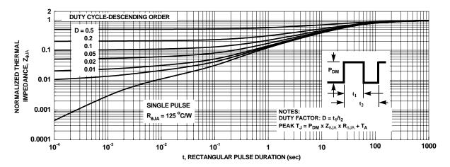
Figure 13. Junction-to-Ambient Transient Thermal Response Curve
