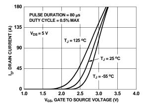
Figure 5. Transfer Characteristics
