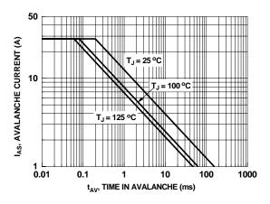
Figure 9. Unclamped Inductive Switching Capability
