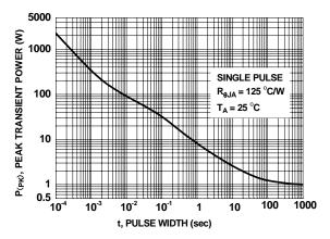
Figure 12. Single Pulse Maximum Power Dissipation
