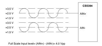
Figure 4. Full Scale Input Voltage
