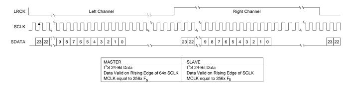
Figure 3. Serial Data Format, DFS High (I<sup>2</sup>S compatible)
