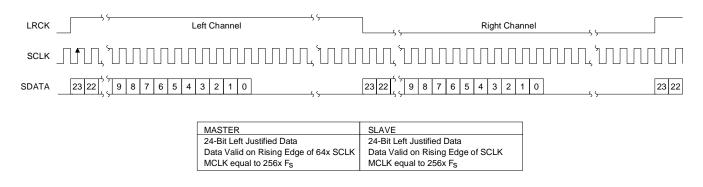
Figure 2. Serial Data Format, DFS Low
