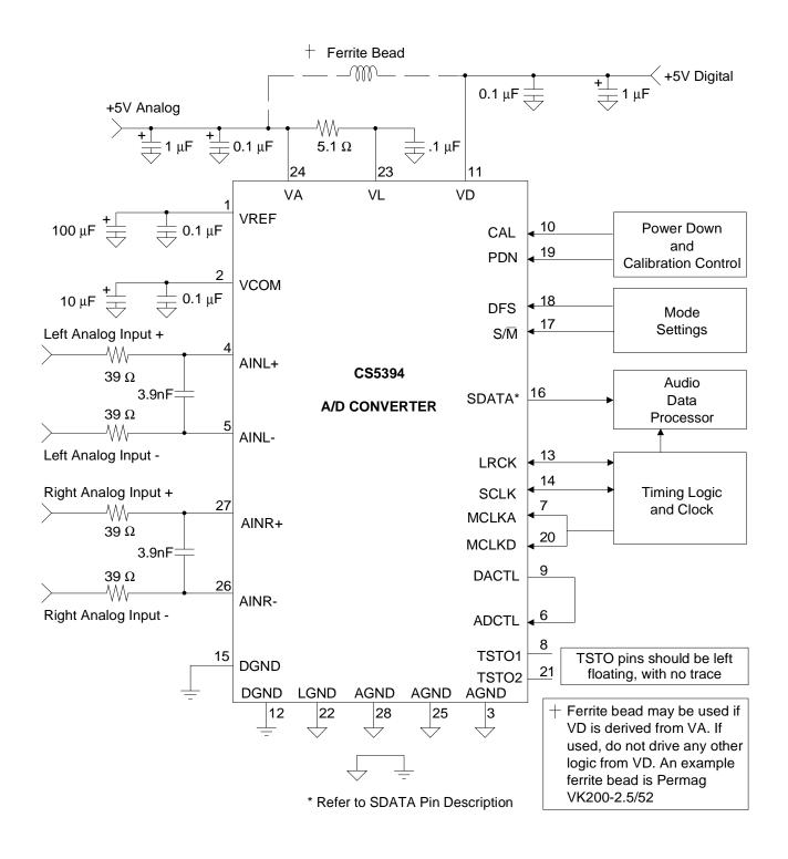
Figure 1. Typical Connection Diagram
