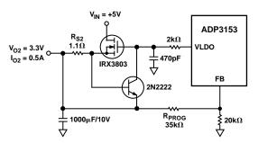
Figure 14. Linear Regulator with Overcurrent Protection
