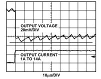
*Figure 10. Transient Response, 1A–14 A of Figure 2 Circuit*
