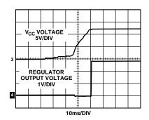
Figure 11. Power-On Start-Up Waveforms
